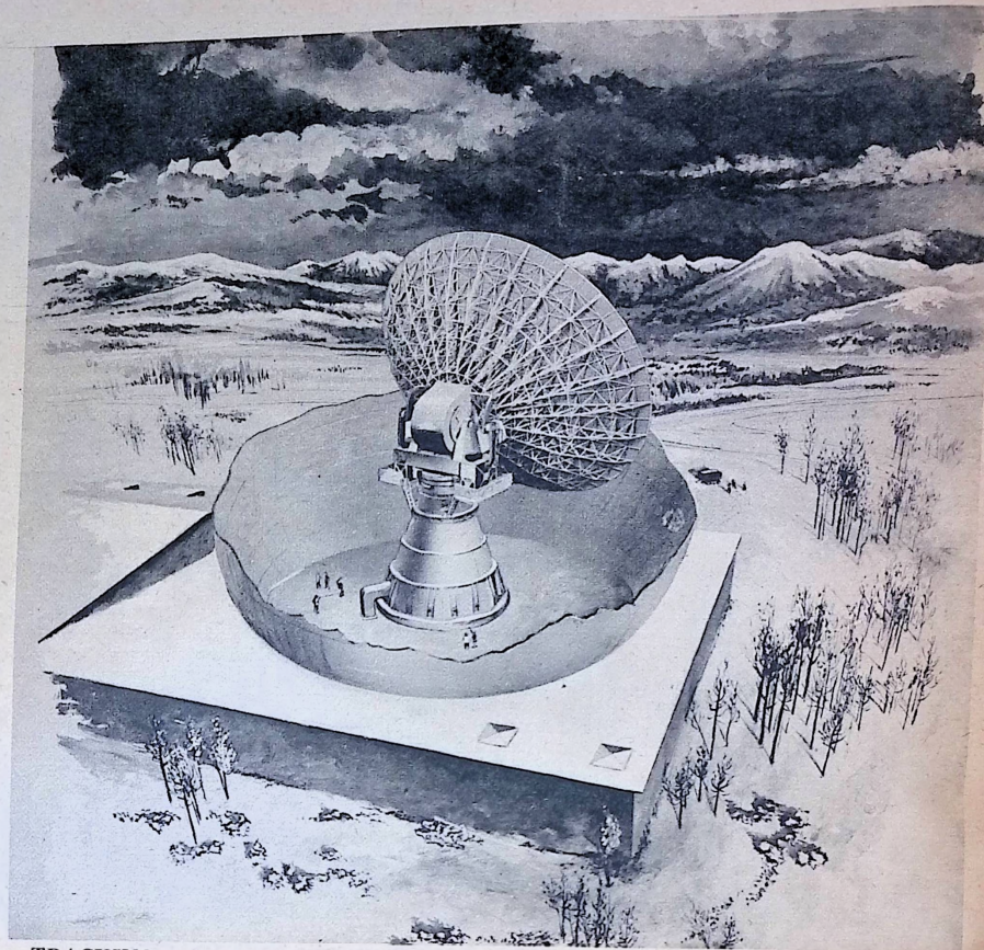
TRACKING RADAR —Artist's cut-away sketch of radar being built by Goodyear Aircraft for R. C. A., prime contractor for Ballistic Missile Early Warning System in Far North. Prototype can be seen from the New Jersey Turnpike ten miles north of Camden.
