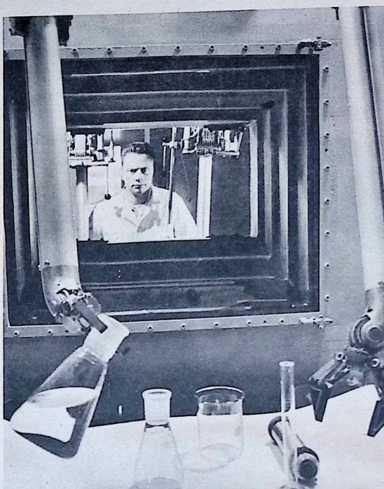
INSIDE A NUCLEAR REACTOR—Shielded by three-foot-thick laminated window, operator at left can perform experiments by remote control. At right is reactor core.
