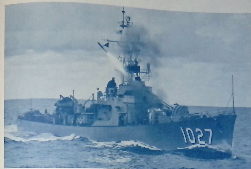
USS JOHN WILLIS, a DEALEY class destroyer escort, fires a rocket powered "weapon Alfa" at a simulated submarine contact during an anti-submarine exercise.
