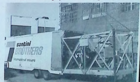
• "Crane Cage" is lowered and leveled with tail gate of trailer for a smooth, swift loading operation.
